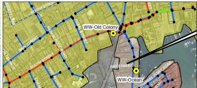
SewerCAD report showing South Street exceeding capacity under future conditions. (Red= flows exceed pipe capacity)
