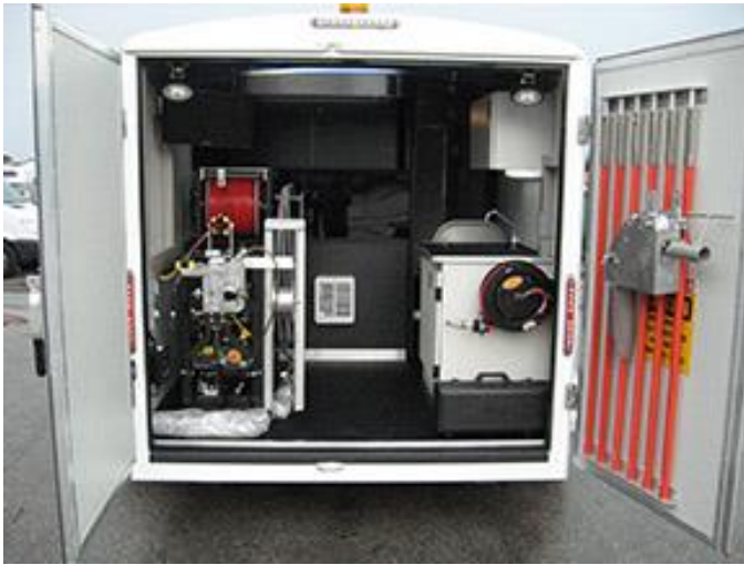
Typical Camera Trailer Setup
