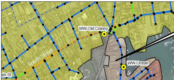
SewerCAD report showing South Street nearing capacity under current conditions (Orange = 15% capacity remaining)
