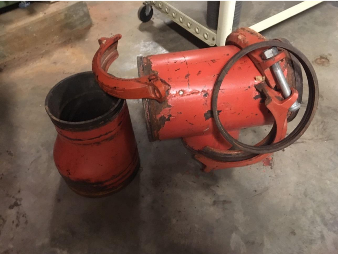
Heating System Victralic Joint
